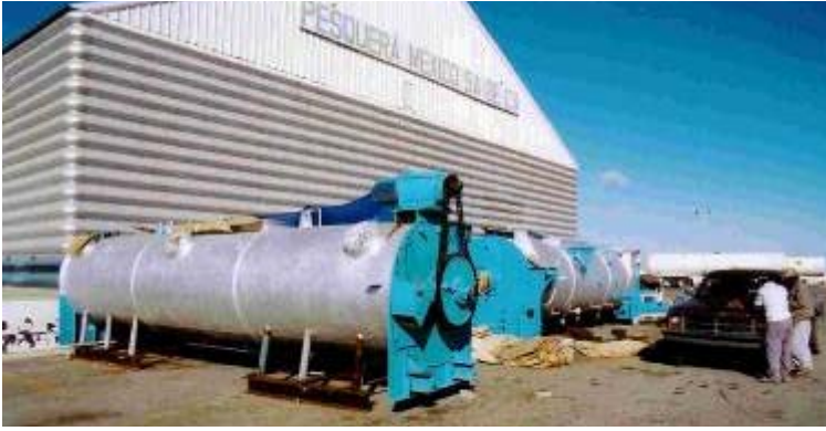
This 60 ton burner has been replaced with a 1000 ton burner. The 60 ton burner has been sold to the Moon plant, creating the capacity to burn 1060 tons per day of sardines for low quality fish meal.
