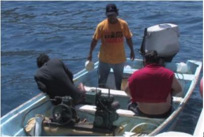
Deadly air: These spear fishermen are using an ancient hookah machine. It's visible on deck in front of the three men. Unless they are maintained regularly, old hookah gear such as this will deliver toxic air to divers
