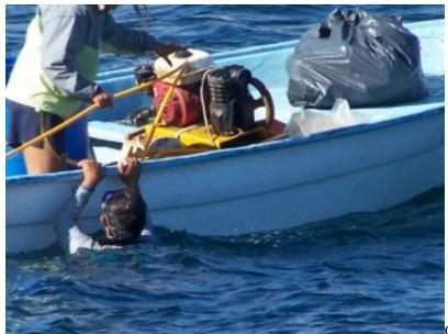
On this boat you can see the hookah gear illegal divers use. It's a small motor that runs an air compressor. The machine feeds air to a diver through a long tube allowing him to stay underwater indefinitely, often at unsafe depths
